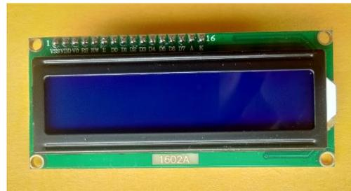
Gambar 7. Liquid Cristal Display
