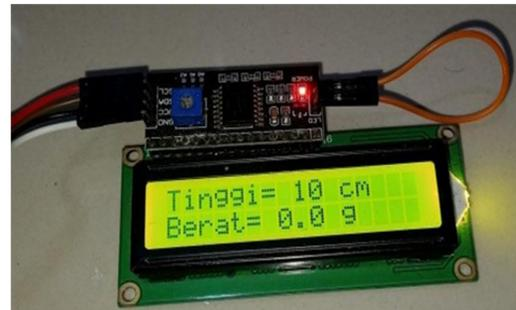
Gambar 15. Liquid Cristal Display
